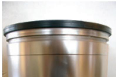
The corrosion resistance of the very hard Lunac 2+ coating is particularly long lasting because unique compressive stresses keep it micro crack free. The coating is well-suited for use in hydraulic systems thanks to its high hardness, anti-cold weld properties and welding quality to the substrate. Lunac 2+ coatings are finished with a roughness of Ra=0.12-0.3µm and do not need any post treatment.
