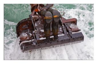
Lunac 2+ duplex successfully combines nearly incompatible characteristics Frequently applied full ceramic piston rod coatings to dredging equipment is often not sufficiently impact resistant. Apart from the outstanding corrosion protection, Lunac 2+ duplex proved to resist most stone chips even without any cracking
