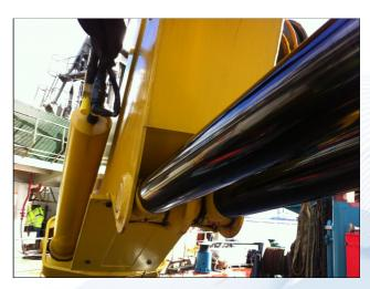
Lunac 2+ duplex applied to hydraulic piston rods, dealing with very hard (mechanical and corrosive) conditions after several years. All preceding coatings failed within 2 years at this spot. These piston rods clearly present the Lunac 2+ dark grey appearance that typically comes along with the Lunac 2+ surface under these harsh conditions.
